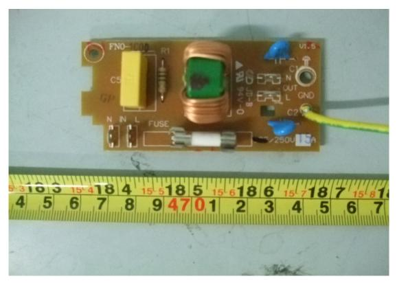
5. Back View of AC Power Filter Board
