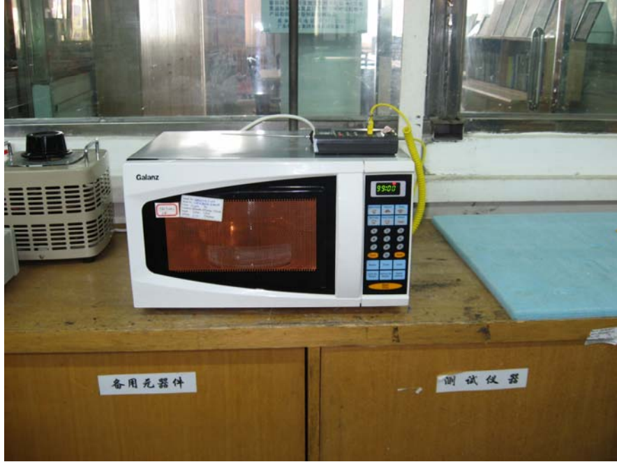
RF Output Power Test Set-Up
