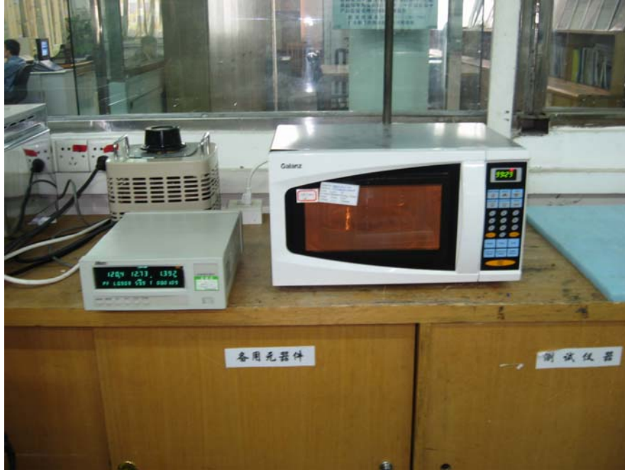
Input Power Test Set-Up
