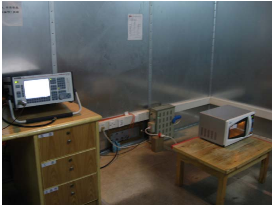
Conducted Emission Test Set-up
