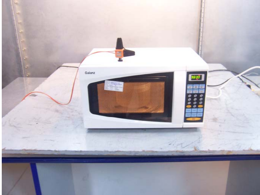
Radiation Hazard Test Set-up
