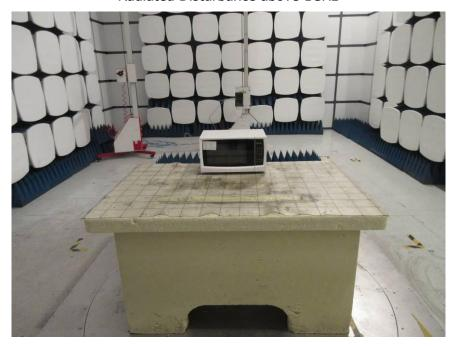
Radiated Disturbance above 9KHz-30MHz
