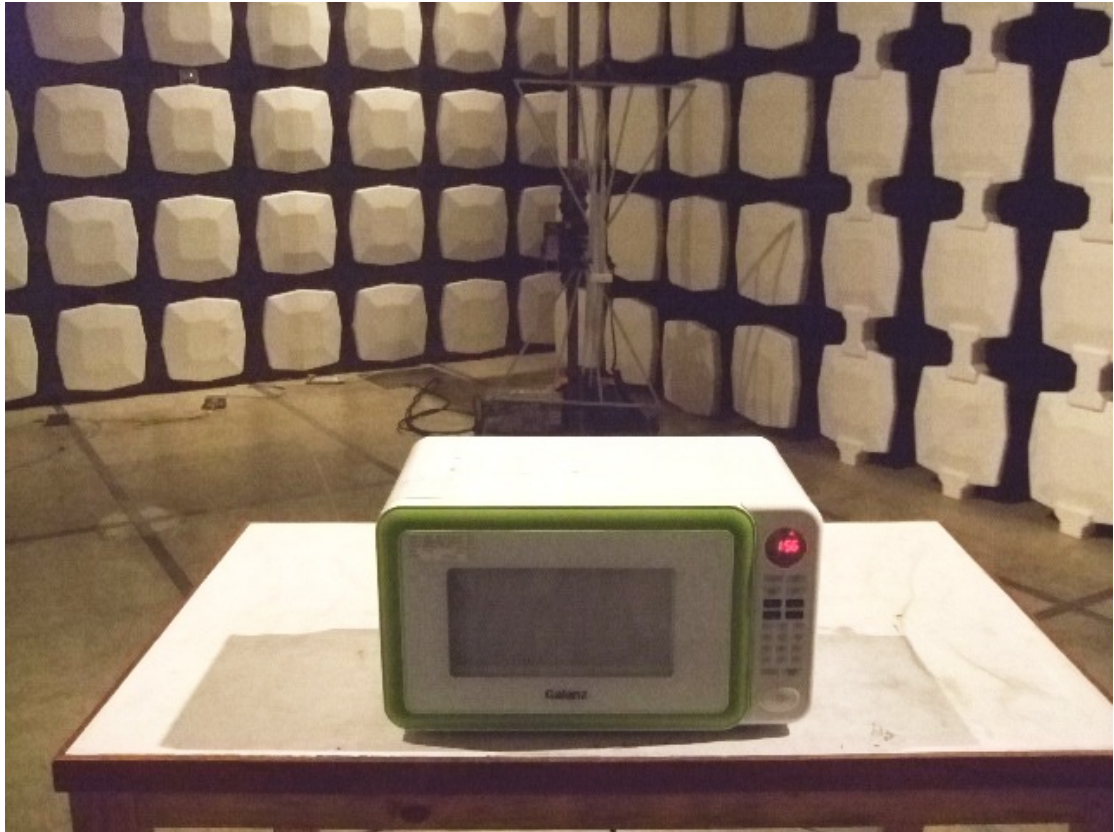
Radiated Emission Test Setup (30-1000MHz)
