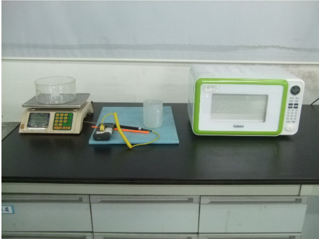
RF Output Power Test Set-up
