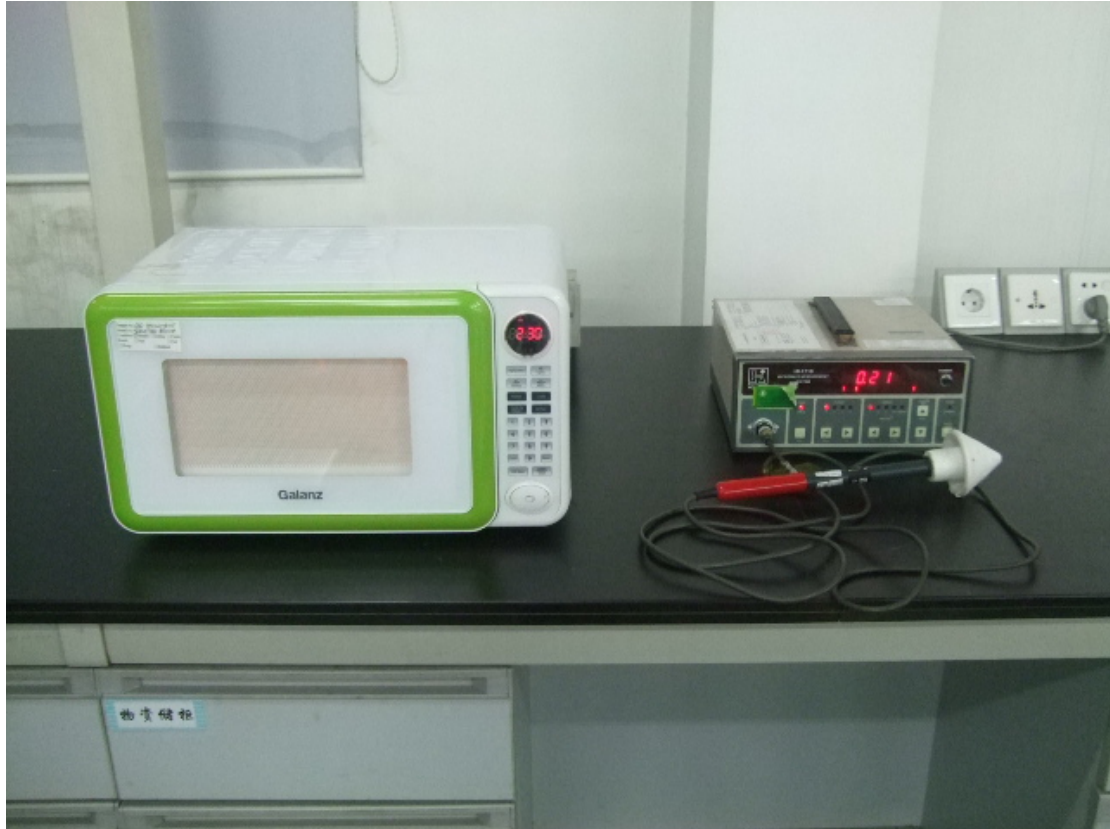
Radiation Hazard Test Setup
