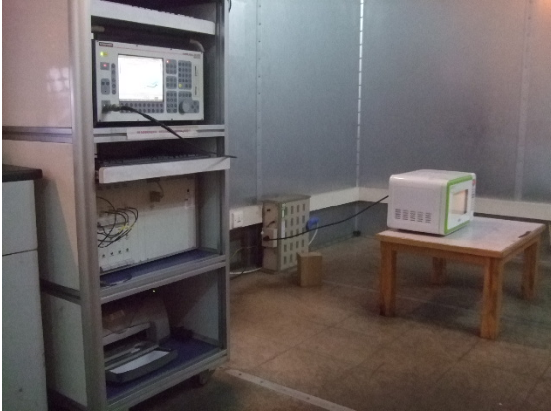
Conducted Emission Test Set-up
