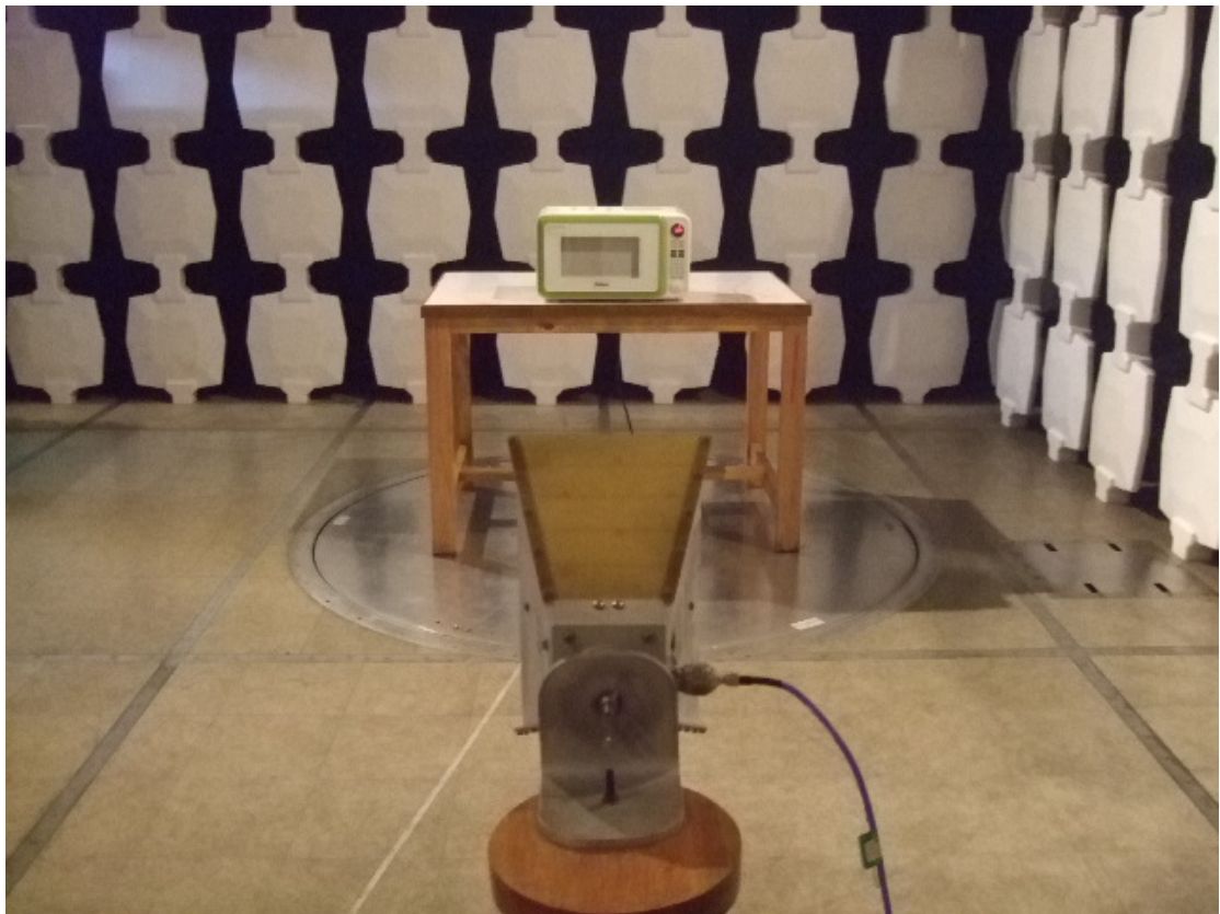
Radiated Emission Test Setup (1-25GHz)
