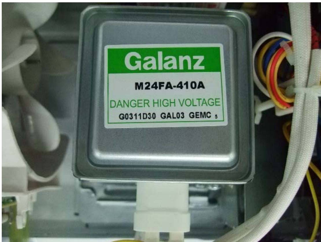
View of Magnetron
