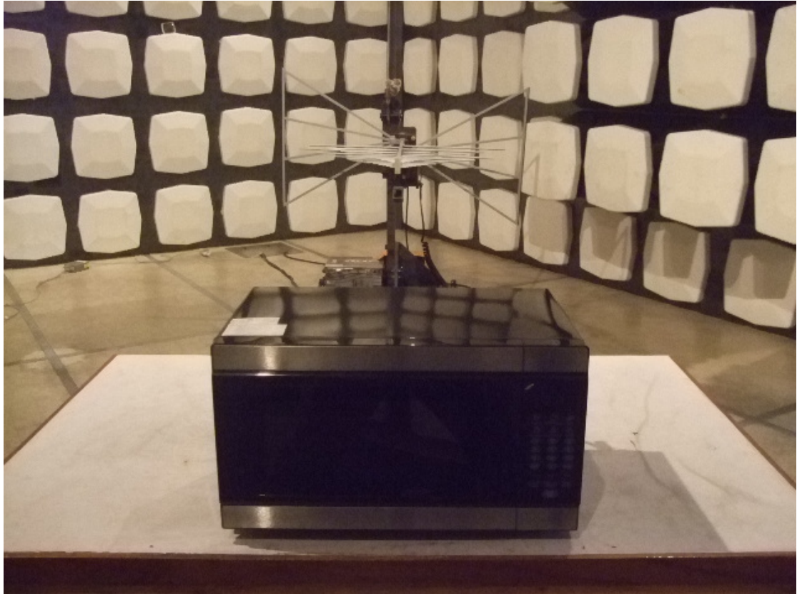
Radiated Emission Test Setup (30-1000MHz)
