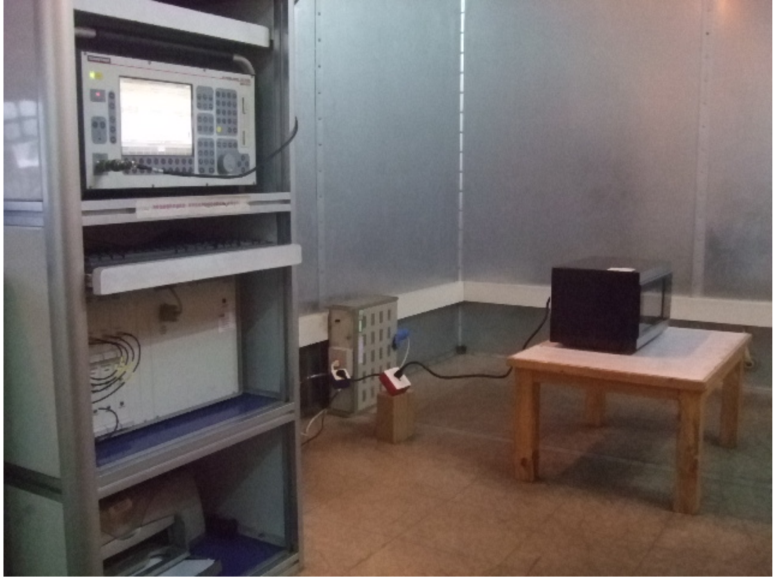
Conducted Emission Test Set-up
