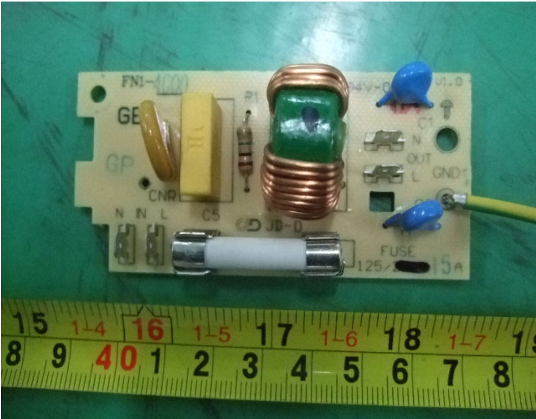
Front View of AC power filter board
