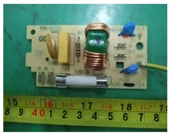
5. Back View of AC Power Filter Board
