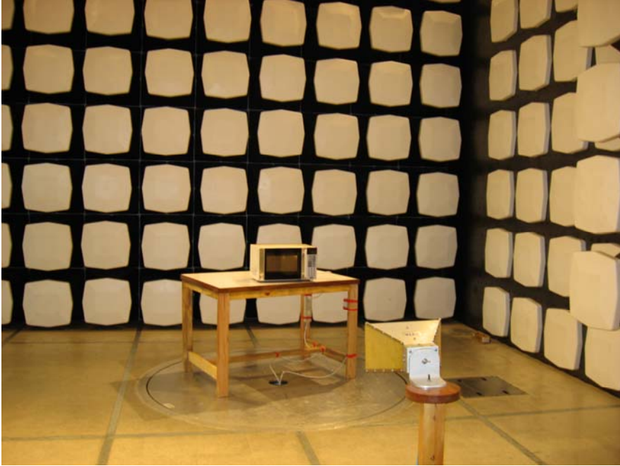
Operating Frequency Test Set-up
