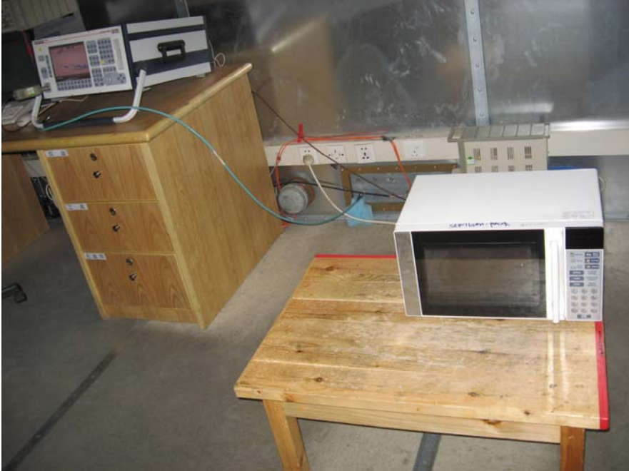
Conducted Emission Test Set-up
