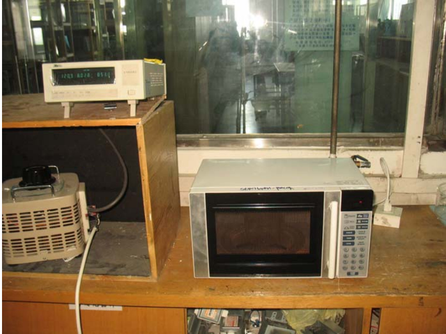
Input Power Test Set-Up
