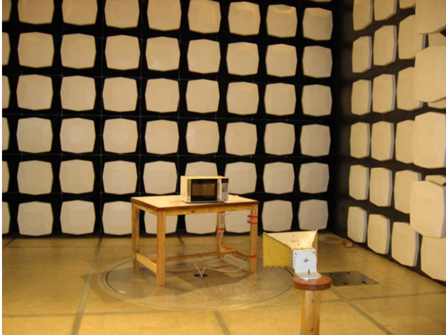
Radiated Emission Test Set-up (1~18GHz)
