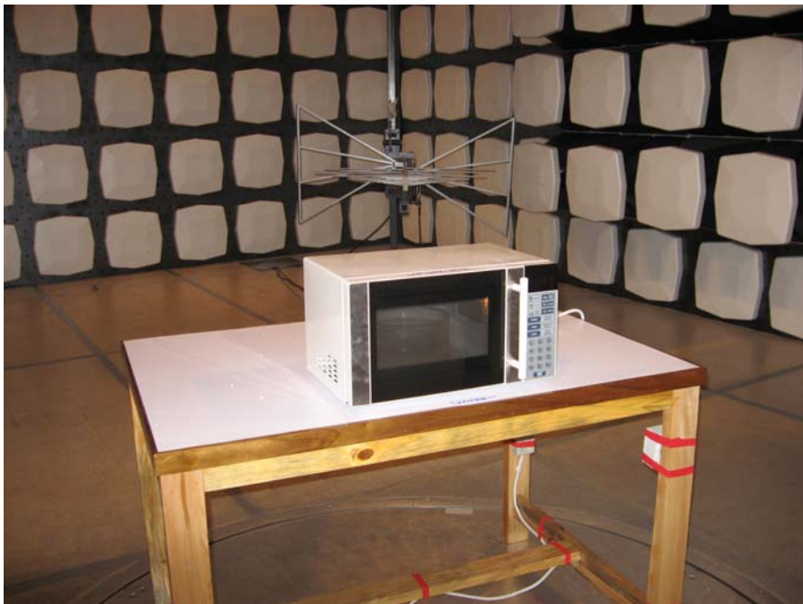
Radiated Emission Test Set-up (30~1000MHz)
