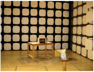
4.Radiated emission measurement
