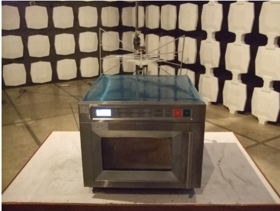
Radiated Emission Test Set-up (30 -1,000MHz)
