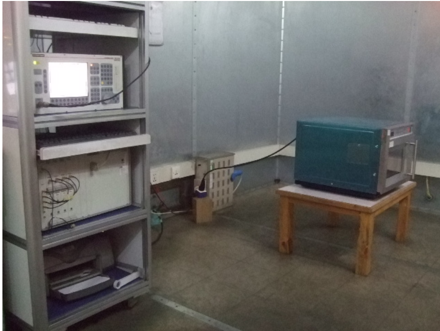
Conducted Emission Test Set-up
