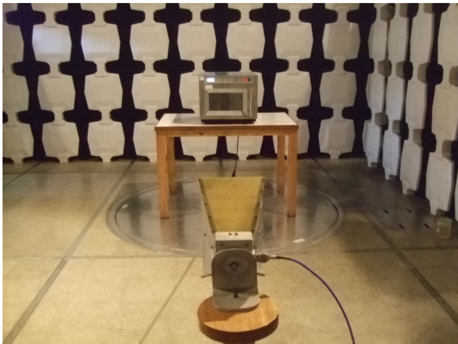
Radiated Emission Test Set-up (1-25GHz)
