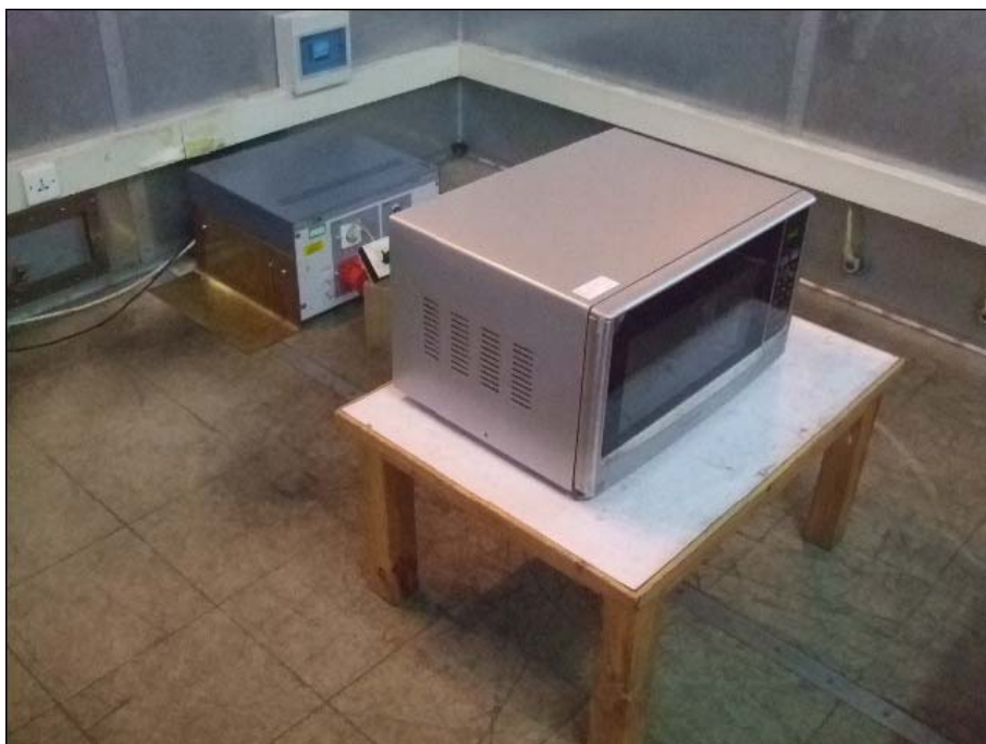
Conducted Emission Test Set-up
