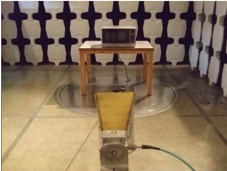
Operating Frequency Test Set-up
