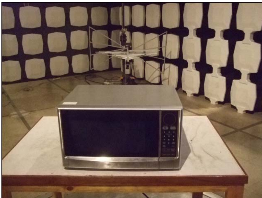
Radiated Emission Test Set-up (30 -1,000MHz)
