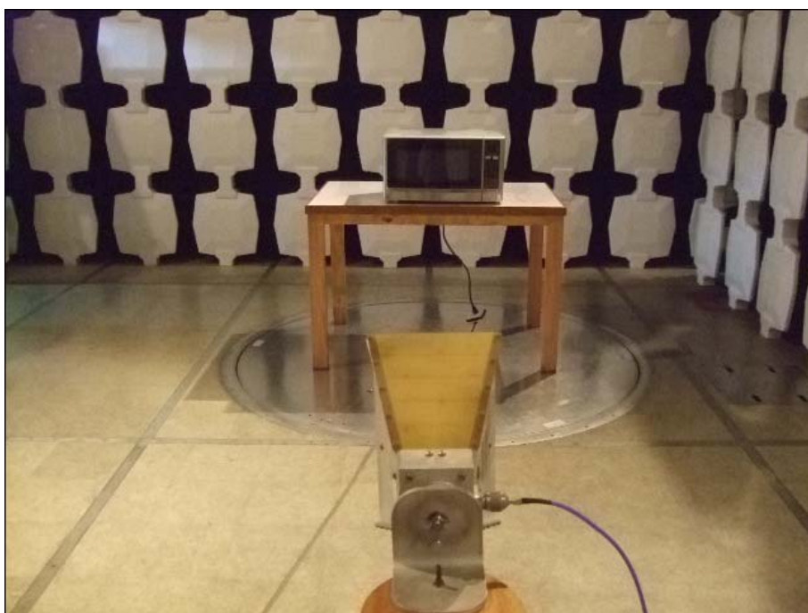
Radiated Emission Test Set-up (1-25GHz)
