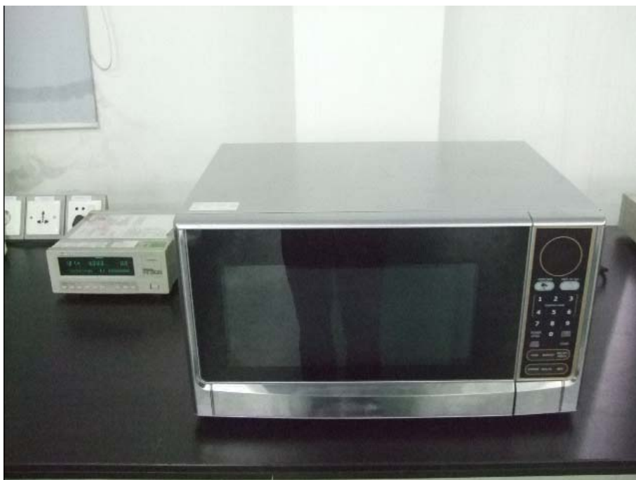
Input Power Test Set-Up
