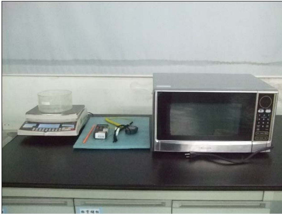
RF Output Power Test Set-Up
