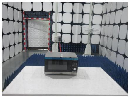
1.6 Radiated Emissions (Magnetic field Strength) (9kHz-30MHz) Test Setup
