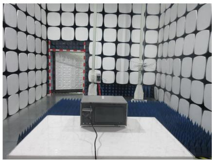
1.4 Radiated Emissions (30MHz-1GHz) Test Setup
