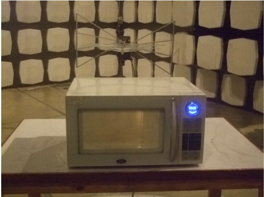
Radiated Emission Test Setup (30-1000MHz)
