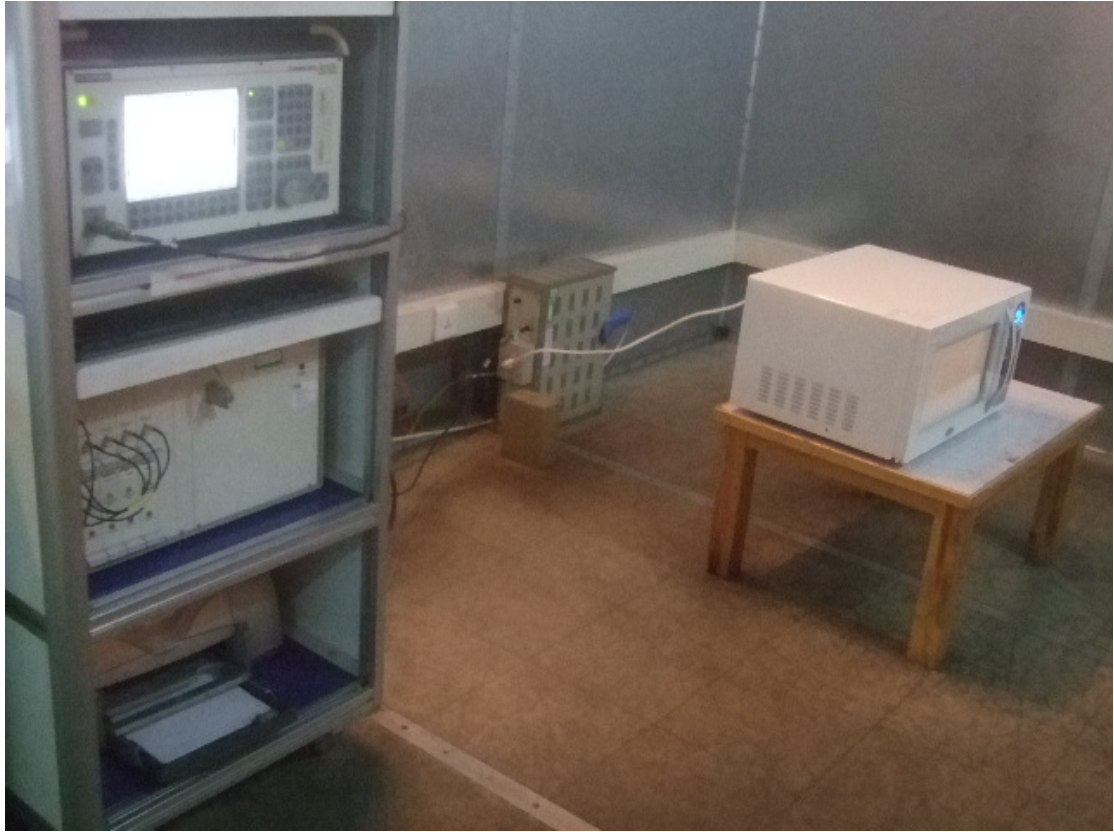
Conducted Emission Test Set-up
