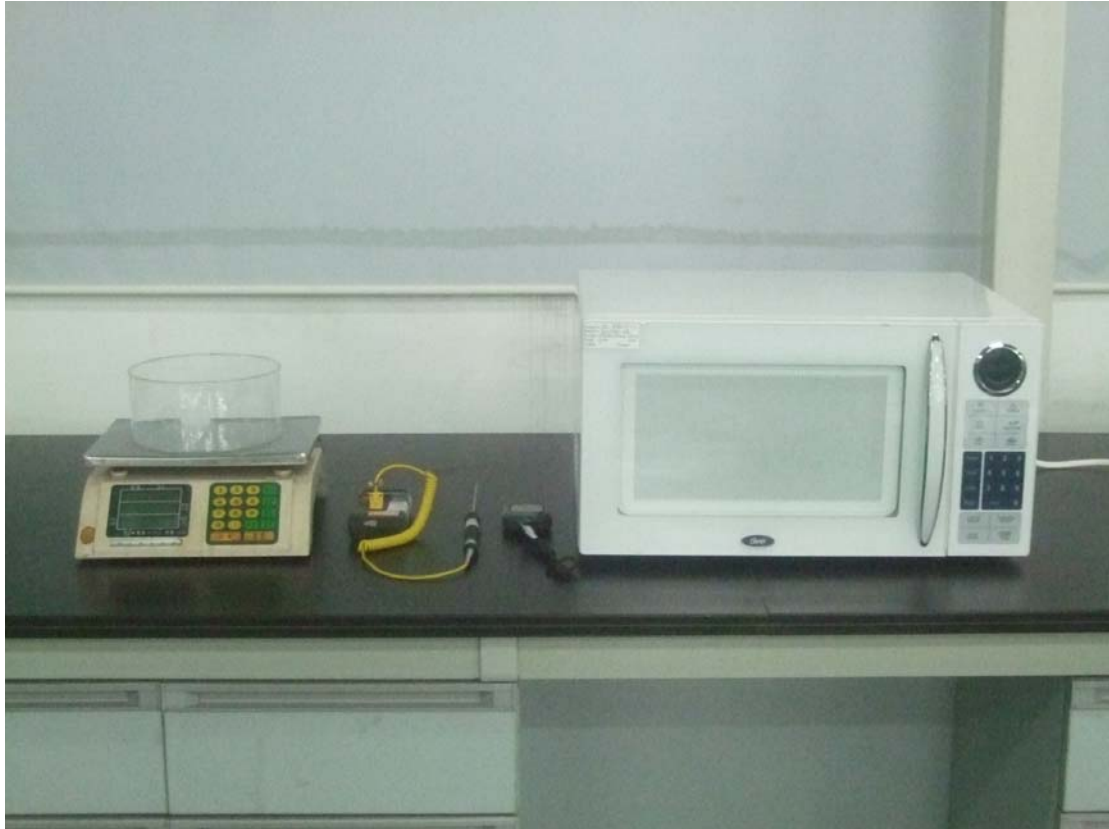
RF Output Power Test Set-up
