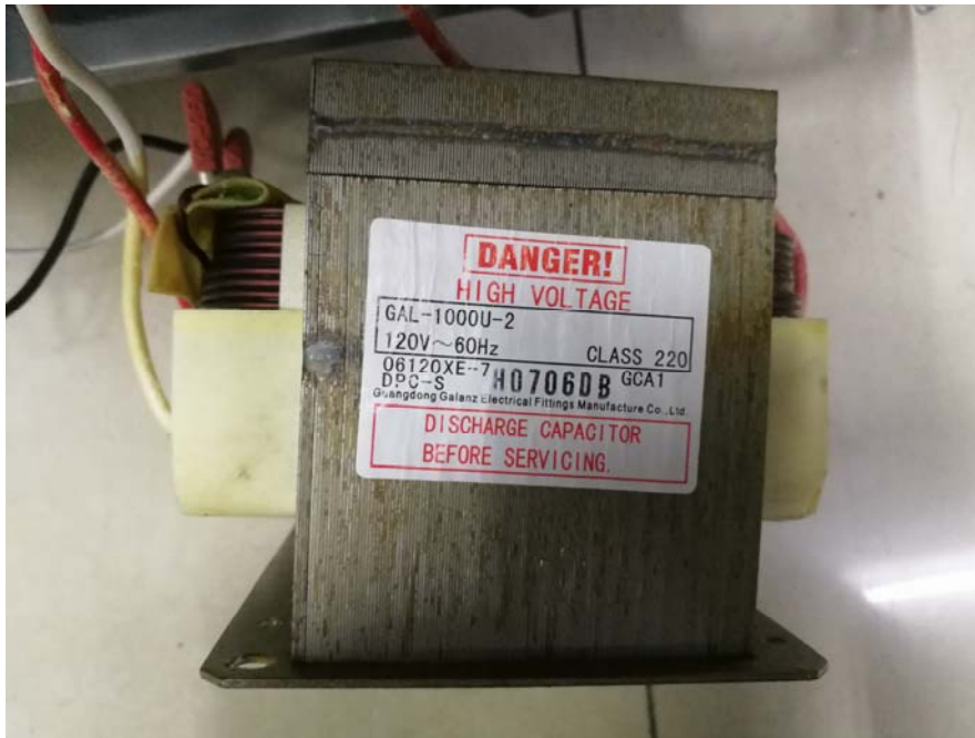
EUT – Transformer View
