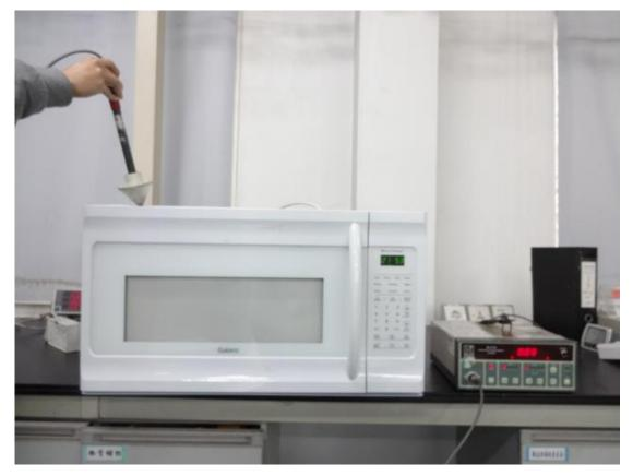
2. Input Power Test Setup
