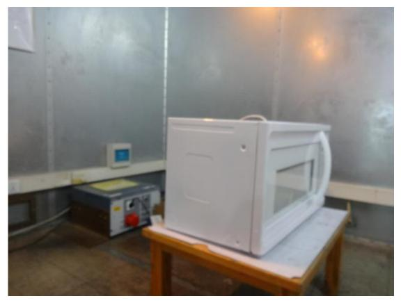
6. Radiated Emission Test Setup
