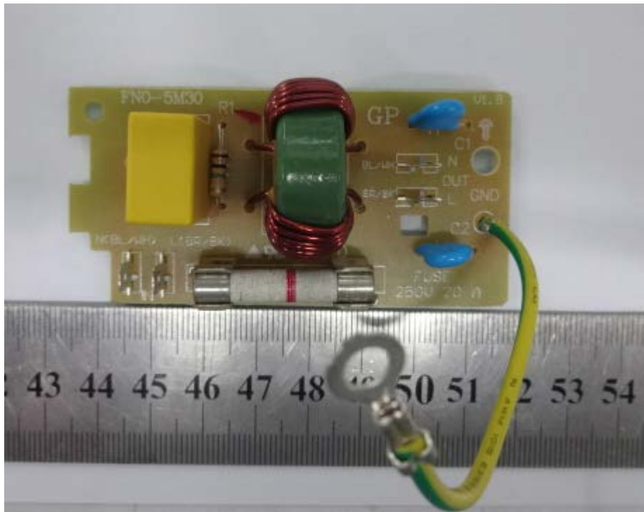
Power Filter Board Top View
