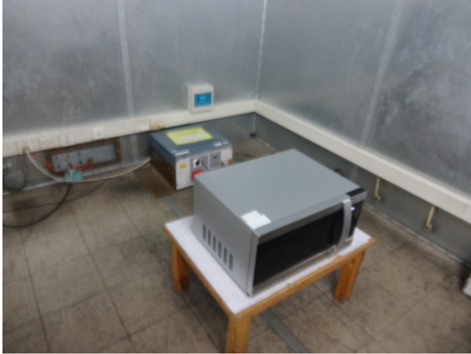
Conducted Emission Test Set-up:
