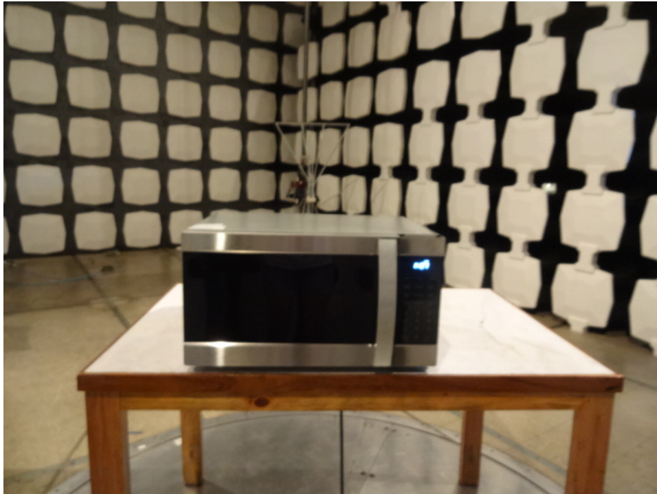
Radiated Emission Test Set-up (30-1000MHz):
