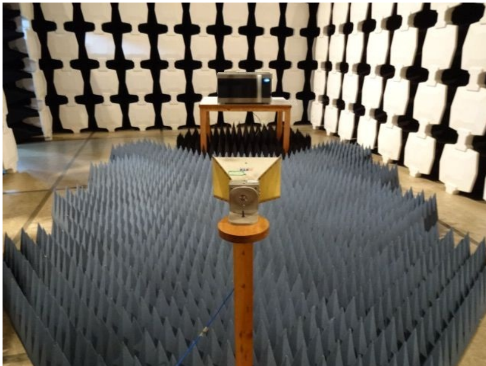
Radiated Emission Test Set-up (1-25GHz):
