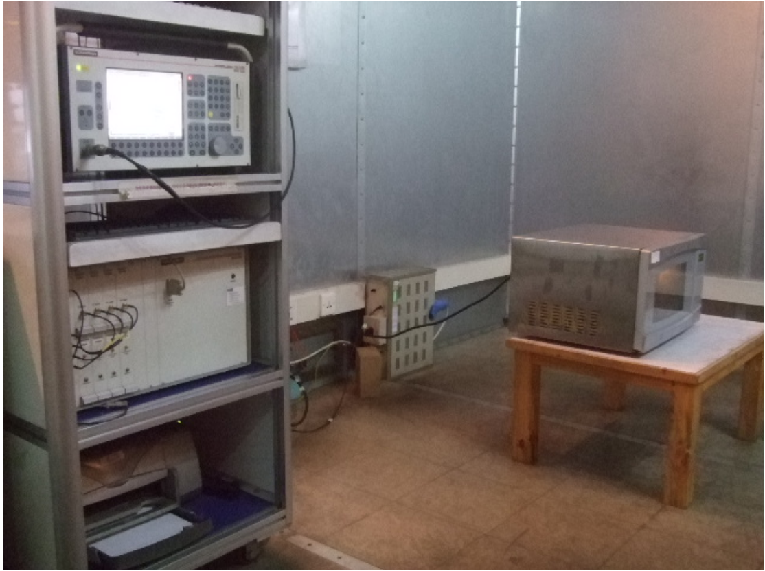
Conducted Emission Test Set-up
