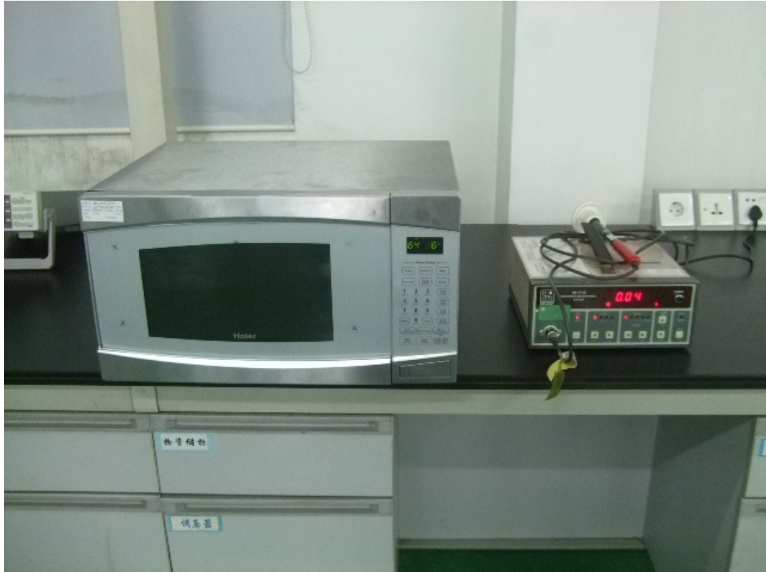
Radiation Hazard Test Setup
