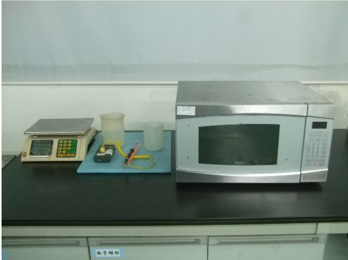
RF Output Power Test Set-up
