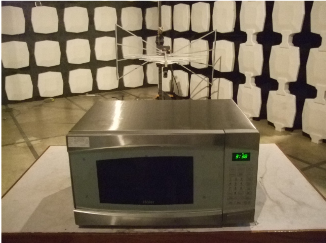
Radiated Emission Test Setup (30-1000MHz)
