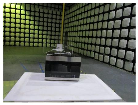
1.4 Radiated Emissions (above 1GHz) Test Setup
