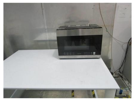
1.2 Radiated Emissions (Magnetic field Strength) (9kHz-30MHz)
