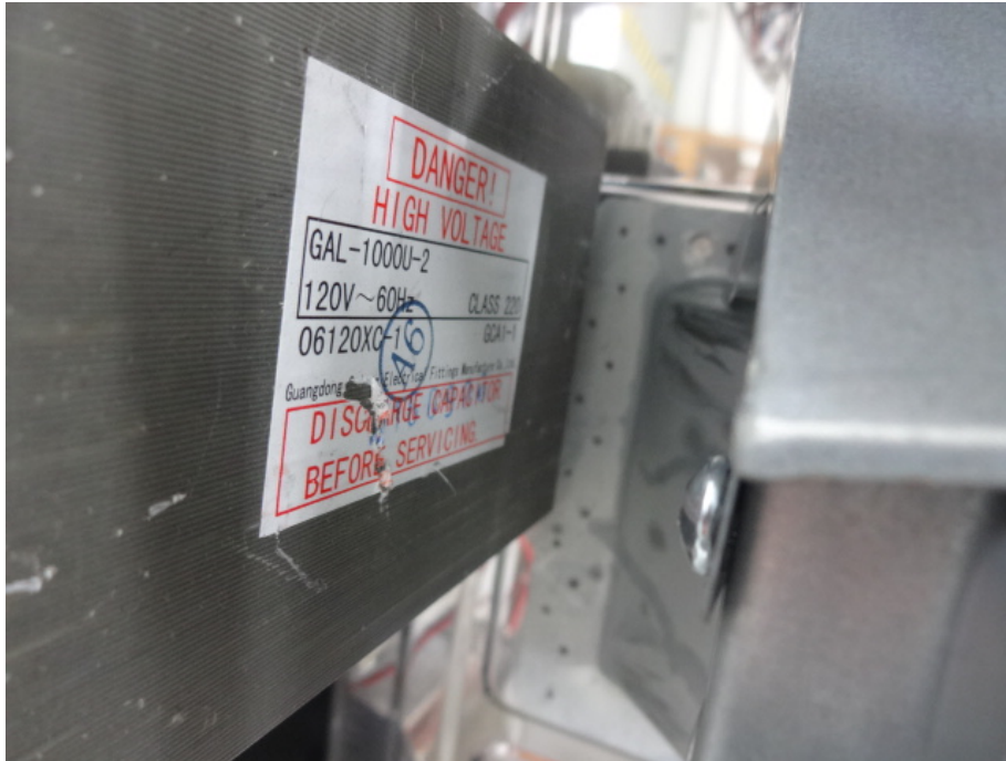
High-voltage Transformer view
