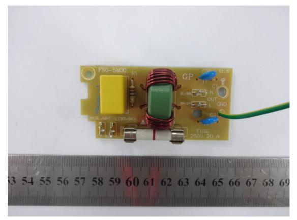
7. Back View of AC Power Filter Board
