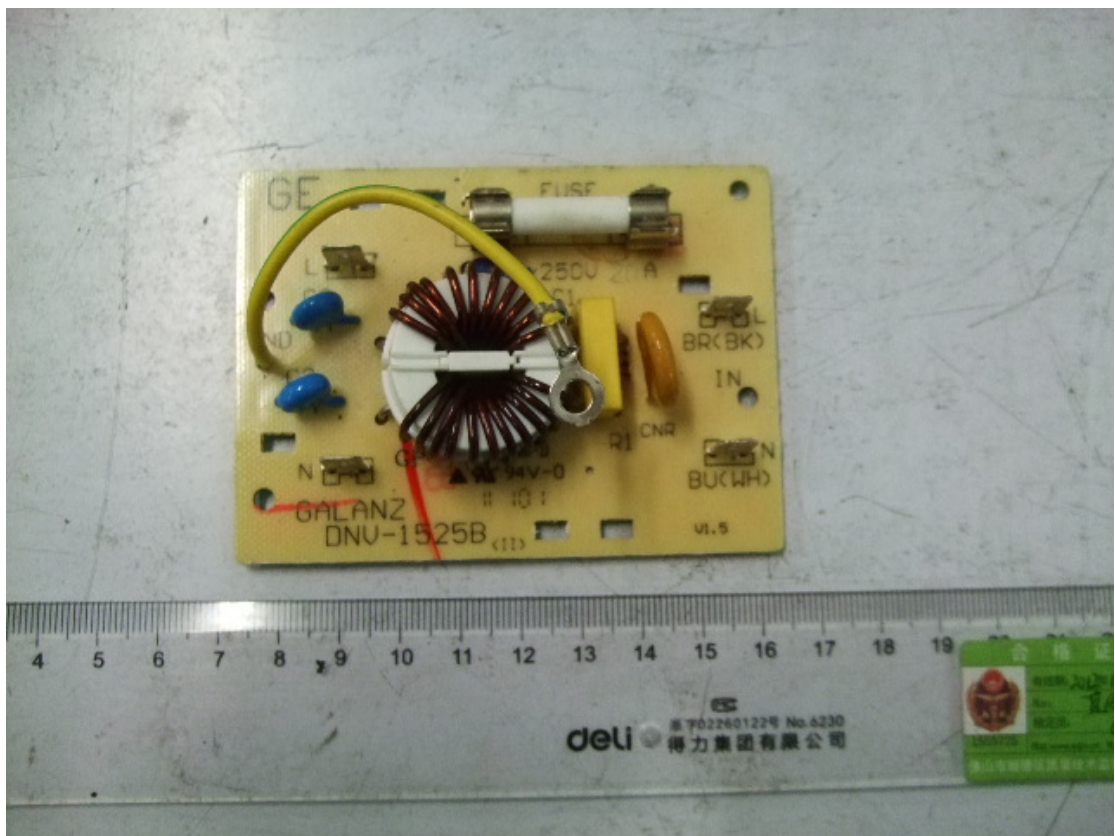
Front View of AC power filter board
