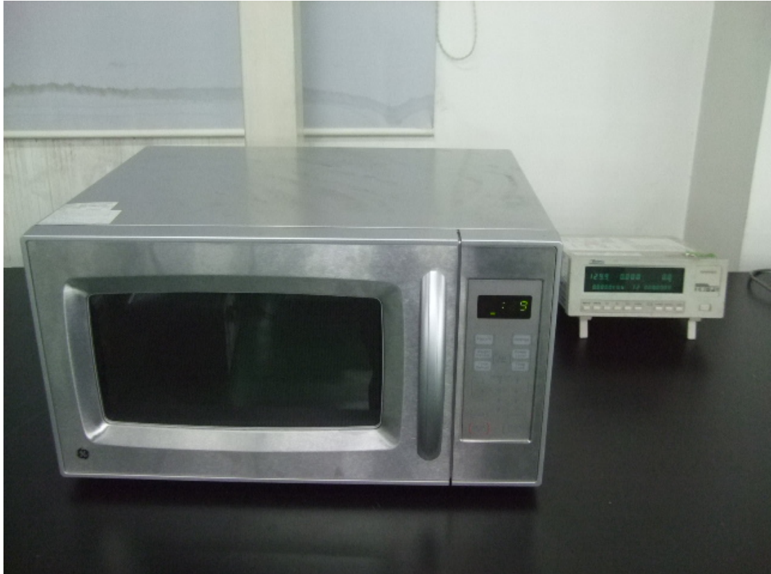
Input Power Test Setup
