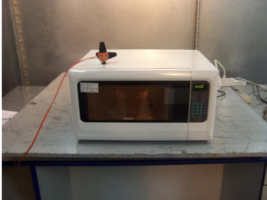
Radiation Hazard Test Set-up
