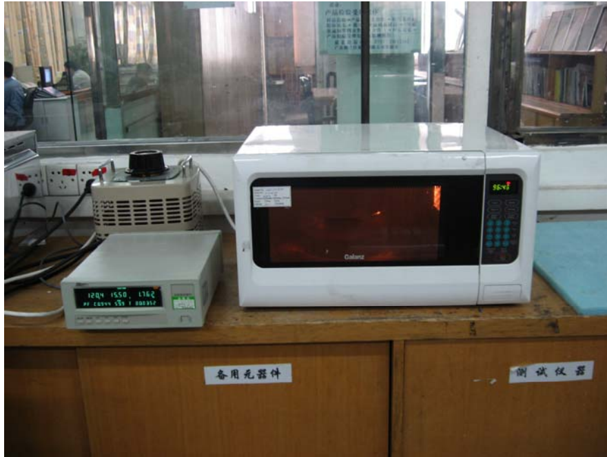
Input Power Test Set-Up
