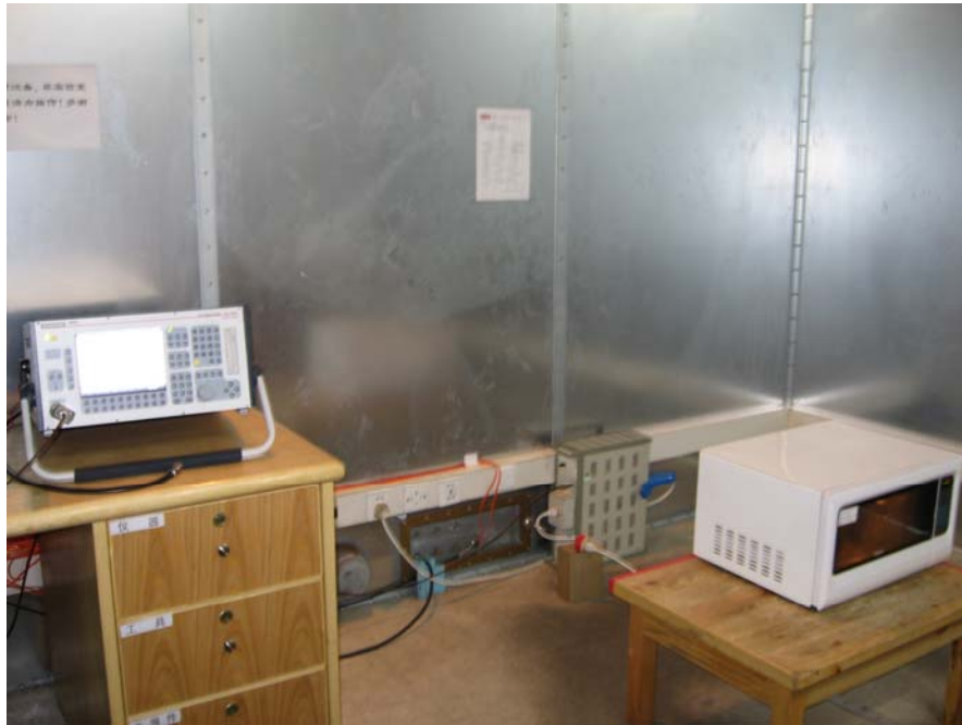
Conducted Emission Test Set-up
