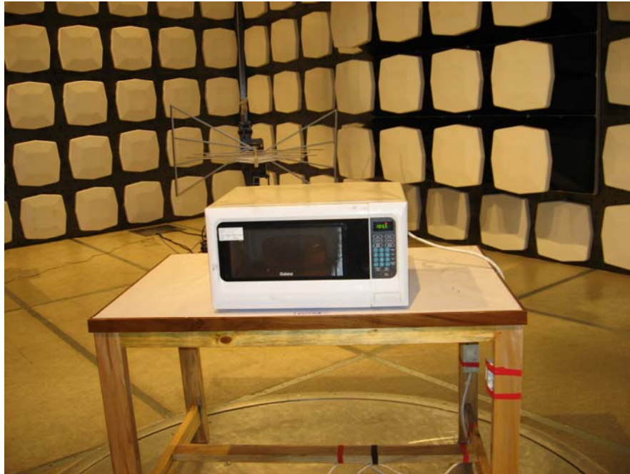
Radiated Emission Test Set-up (30~1000MHz)
