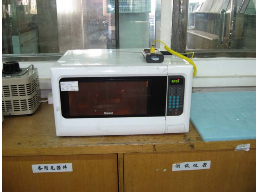
RF Output Power Test Set-Up
