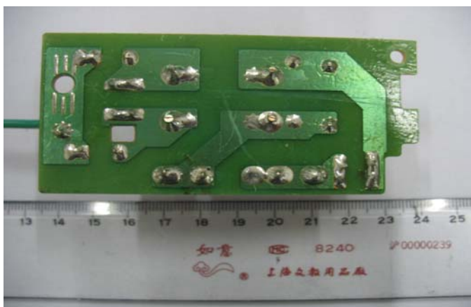
Photo 3 - Back view of AC Power filter board
