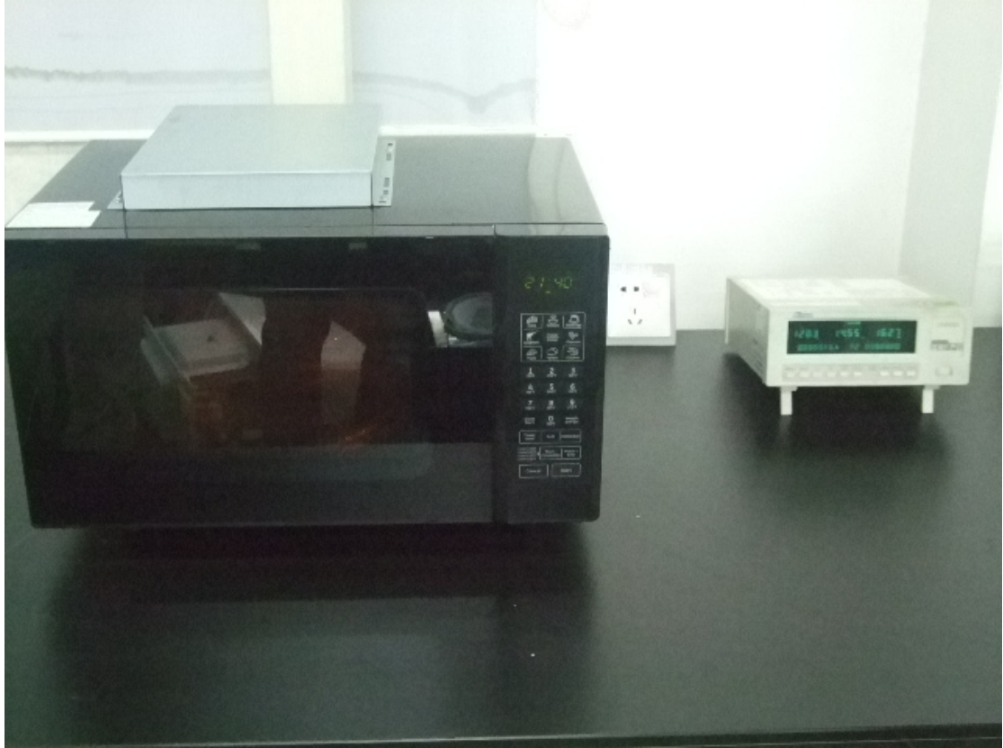
Input Power Test Setup
