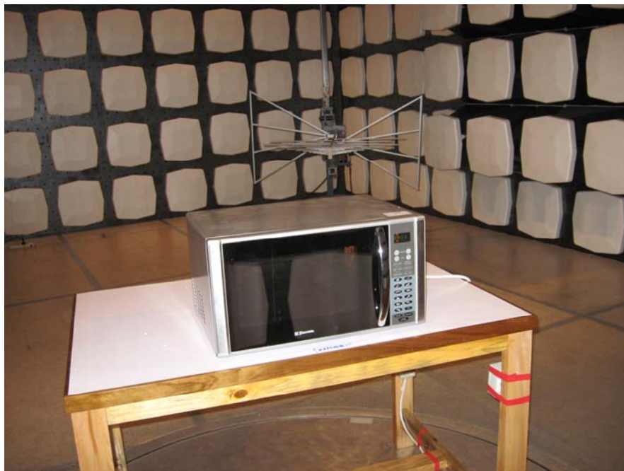
Radiated Emission Test Set-up (30~1000MHz)
