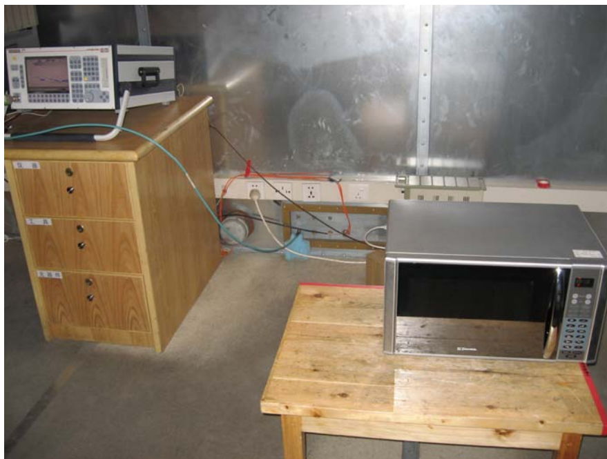
Conducted Emission Test Set-up
