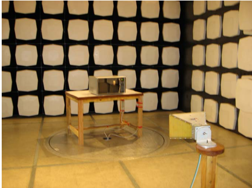
Radiated Emission Test Set-up (1~18GHz)
