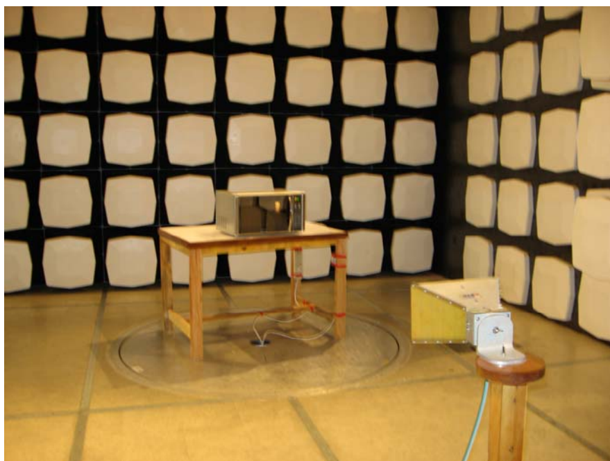
Operating Frequency Test Set-up
