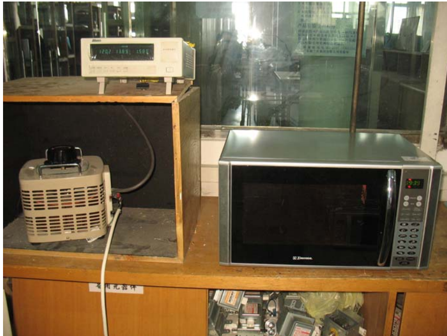
Input Power Test Set-Up
