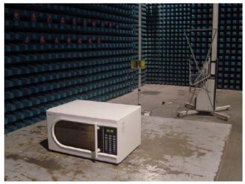
4. Radiated emission measurement
