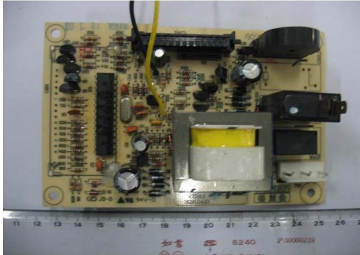
Photo 3 –Front view of Main board
