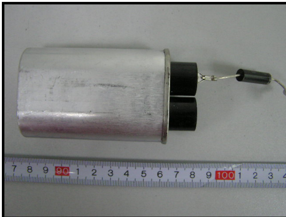
EUT- High Capacitor Rear View
