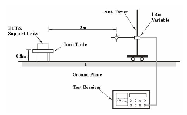
The radiated emission tests were performed in the 3 meters chamber A test site, using the setup accordance with the FCC MP - 5. The specification used was the FCC part 18.
