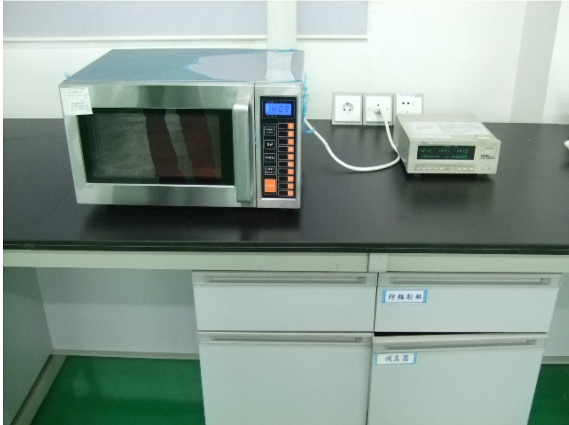
Input Power Test Setup
