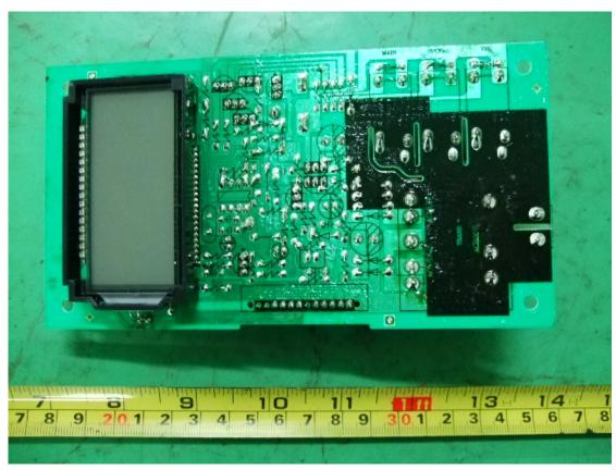
4. Front View of AC Power Filter Board
