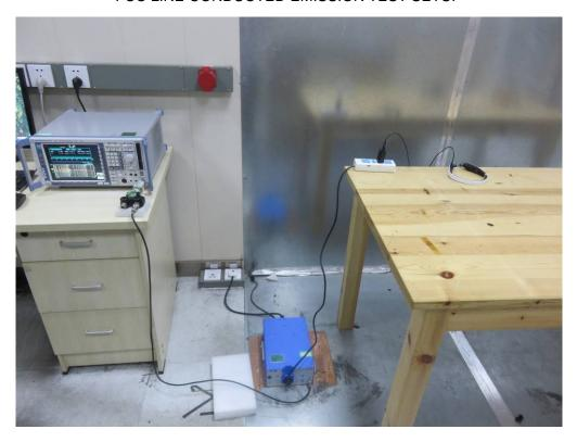
FCC RADIATED EMISSION TEST SETUP
