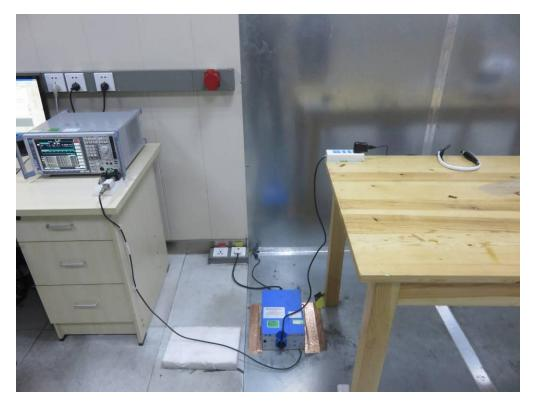
FCC RADIATED EMISSION TEST SETUP
