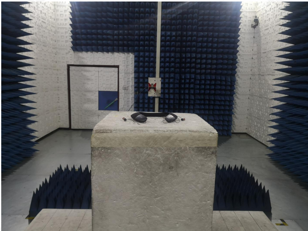
RADIATED EMISSION TEST SETUP ABOVE 1GHZ
