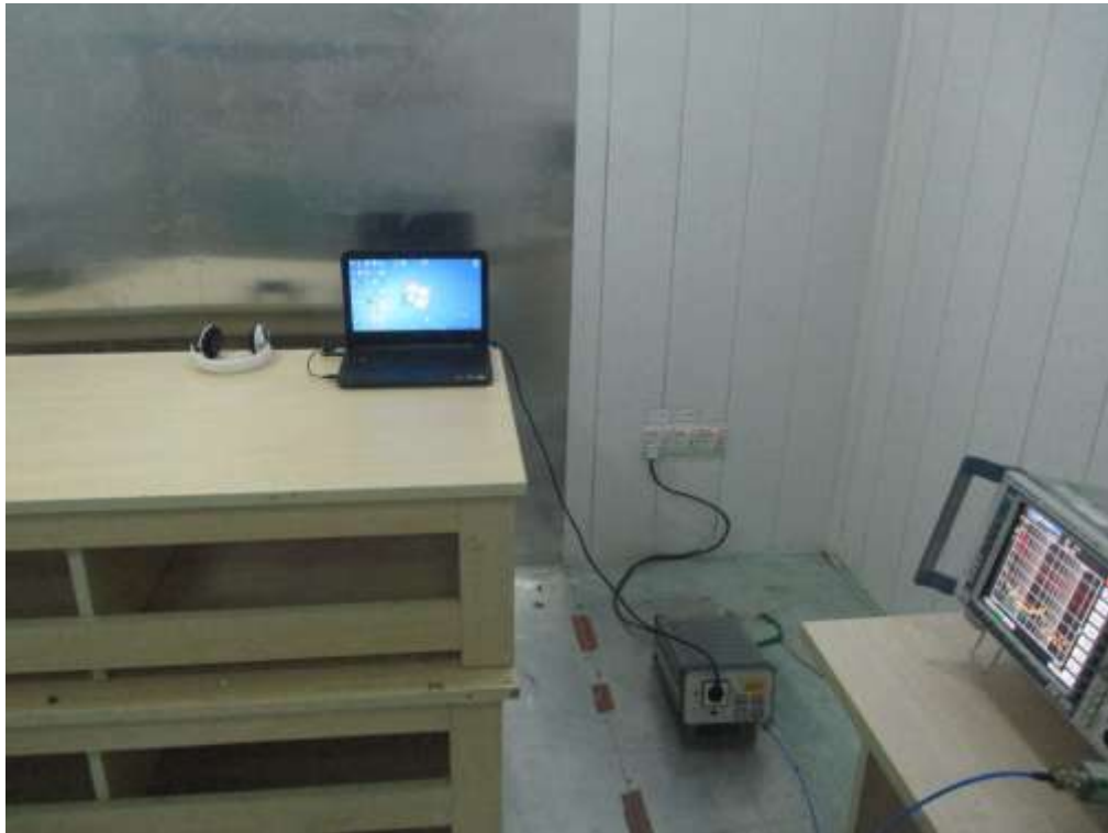
FCC RADIATED EMISSION TEST SETUP
