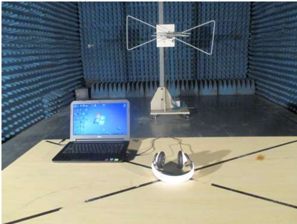
FCC RADIATED EMISSION TEST SETUP
