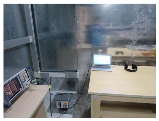
FCC RADIATED EMISSION TEST SETUP
