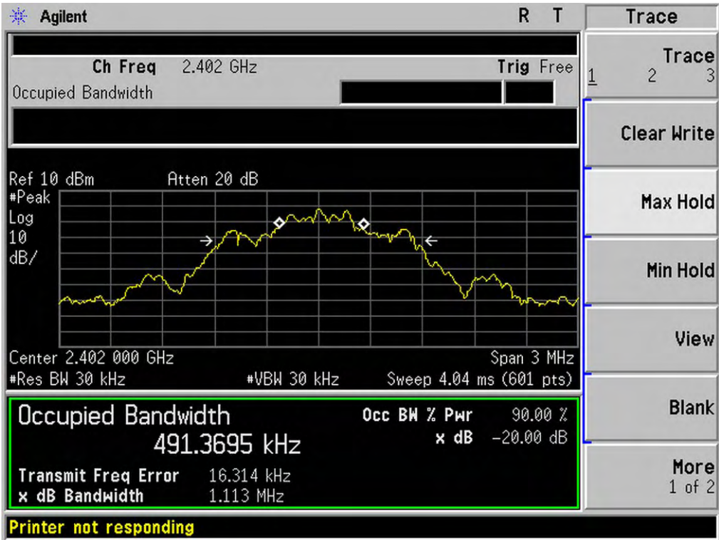
TEST PLOT OF BANDWIDTH FOR LOW CHANNEL
