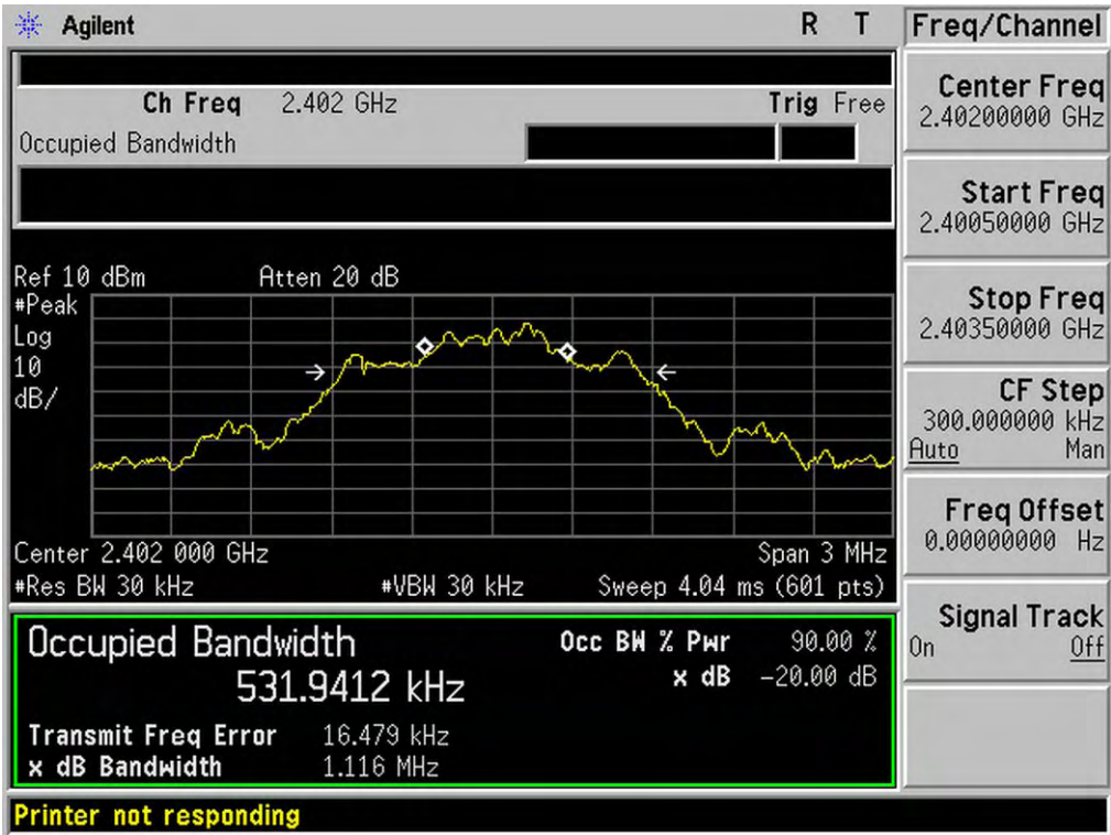
TEST PLOT OF BANDWIDTH FOR LOW CHANNEL
