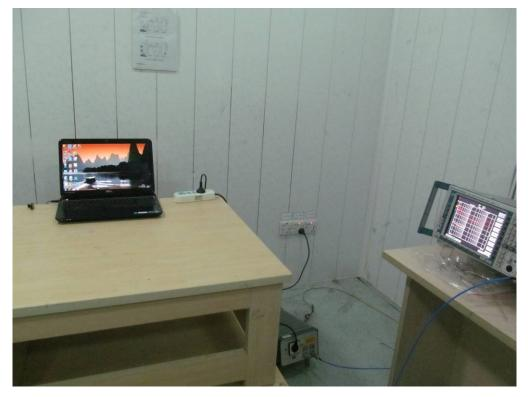
FCC RADIATED EMISSION TEST SETUP
