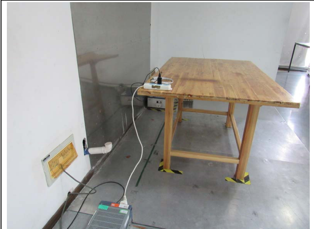
Conducted Emissions Test Setup Side View
