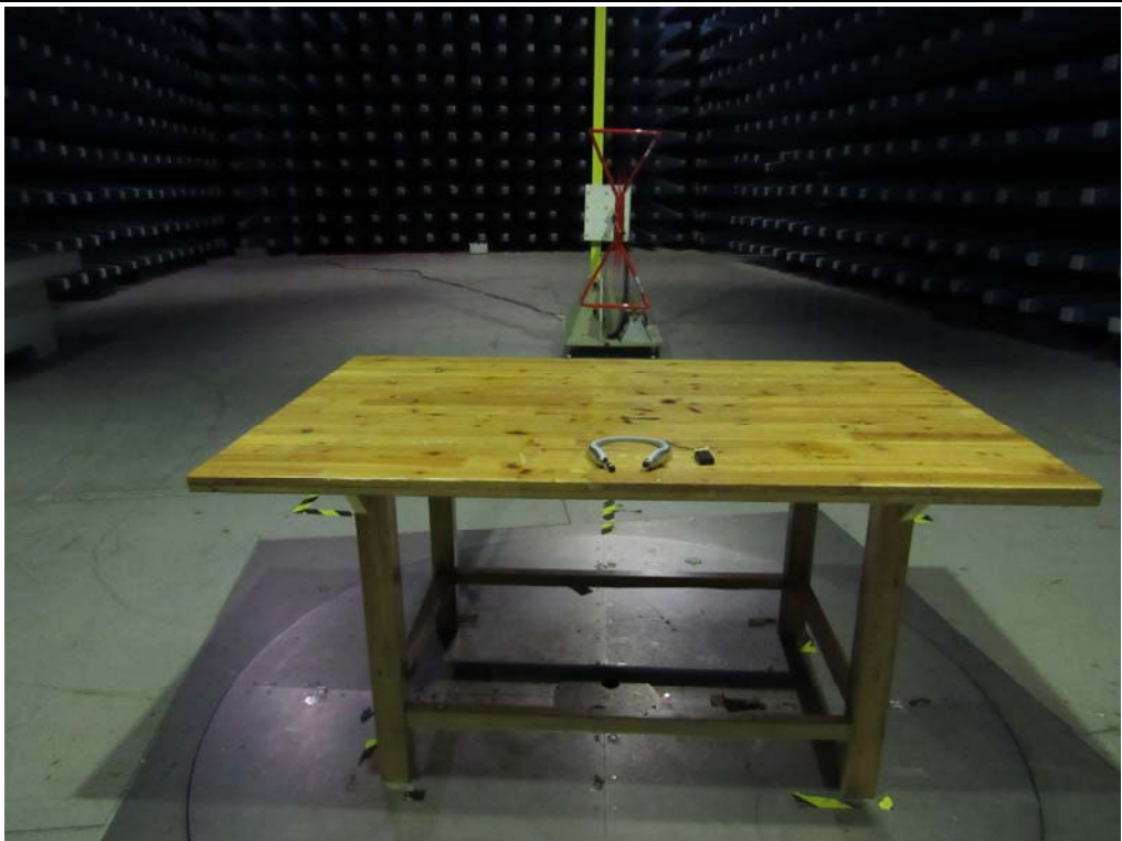
Radiated Spurious Emissions Test Setup Below 1GHz Rear View
