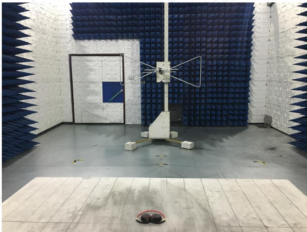
RADIATED EMISSION TEST SETUP ABOVE 1GHZ
