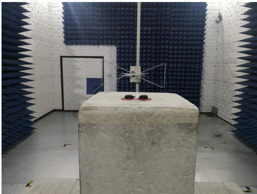
RADIATED EMISSION TEST SETUP ABOVE 1GHZ
