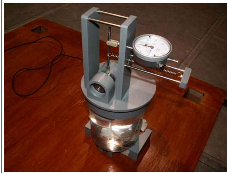
Strength test equipment, implant placed in saline solution to simulate human body.
