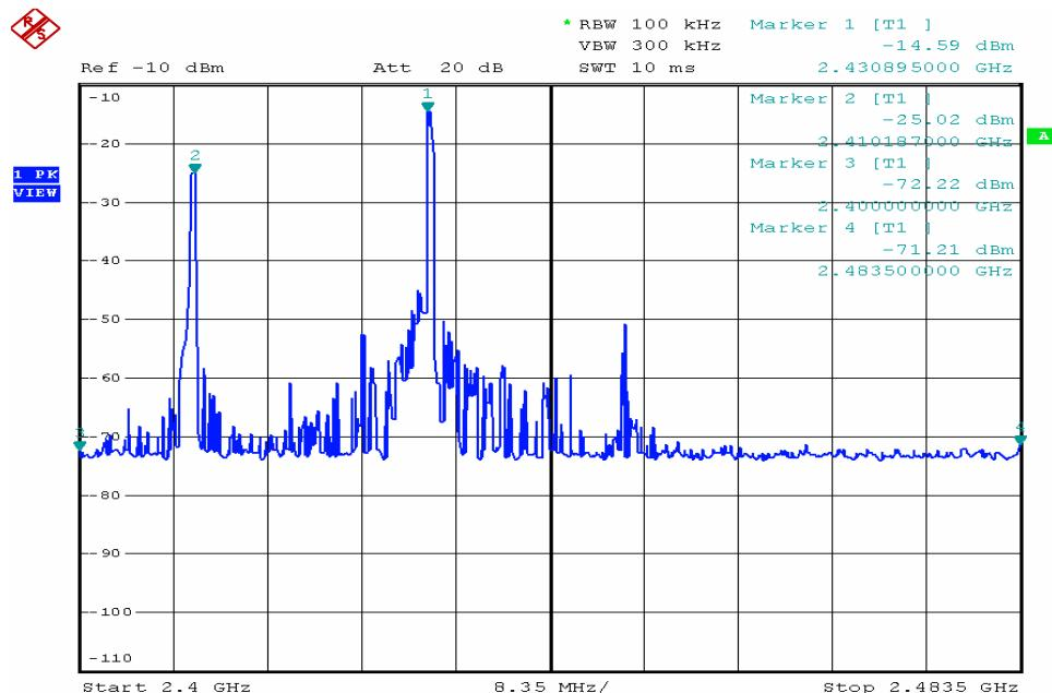
The test result for the Emissions radiated outside of the specified frequency bands , please refer the section 5.3.1 of this report.
