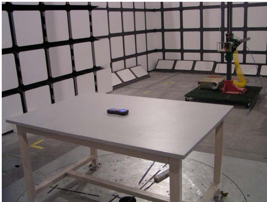
Radiated Emissions - Rear View (Above 1 GHz)
