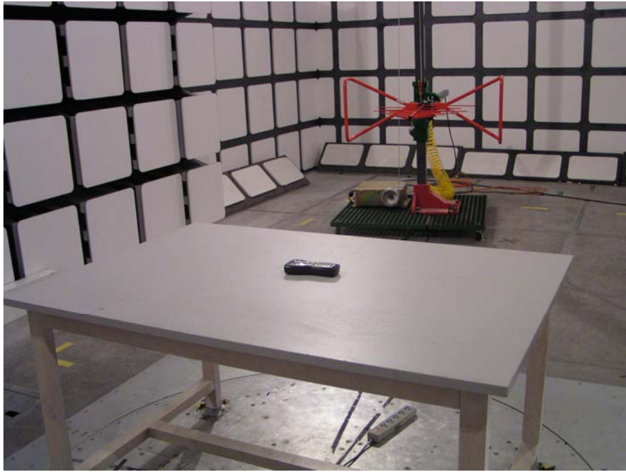
Radiated Emissions - Front View (30 MHz-1 GHz)
