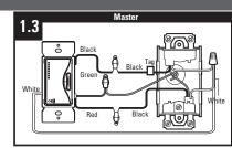
Connect master dimmer as shown by connecting black wire of dimmer to tagged "Hot" wire. Red wire must be connected to the wire that goes to the light.
