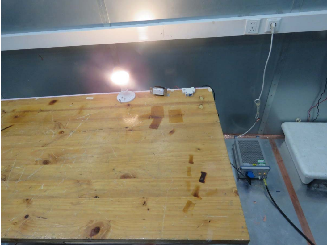
Picture 2 Conducted Emission Test Setup
