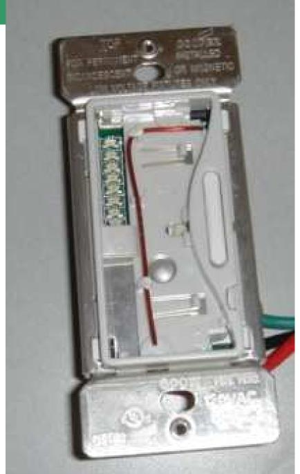
RF Dimmers Typical Antenna placement
