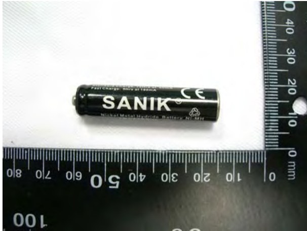
Figure 2. Battery (Ni-MH 1.2V × 2 , 600mAh)
