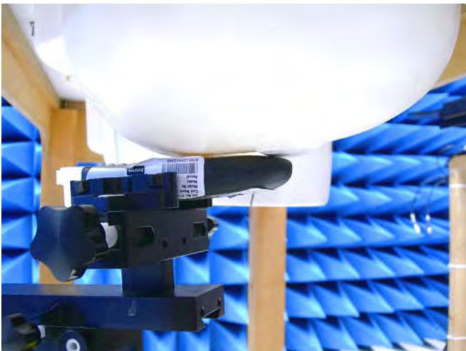
Figure 16. Left Head SAR Test Setup (Cheek)
