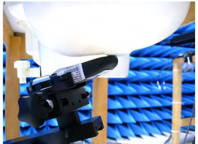
Figure 17. Left Head SAR Test Setup (Tilted)
