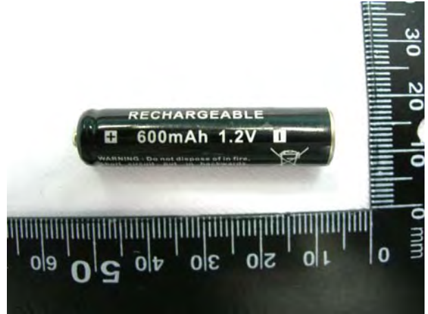
Figure 2. Battery (Ni-MH 1.2V × 2 , 600mAh)
