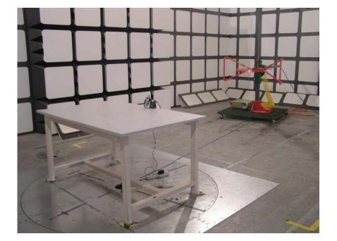
Charging Mode: Radiated Emission - Rear View (30-1000MHz)
