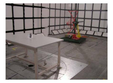
Radiated Emission - Rear View (30-1000MHz)
