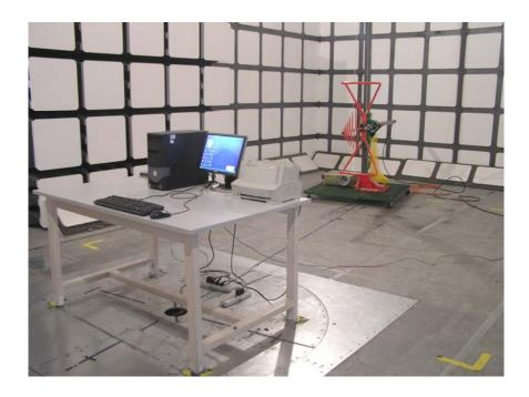
Radiated Emission – Rear View (30-1000MHz)
